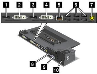
**1 3 DisplayPort connector**: Connect a display device.
